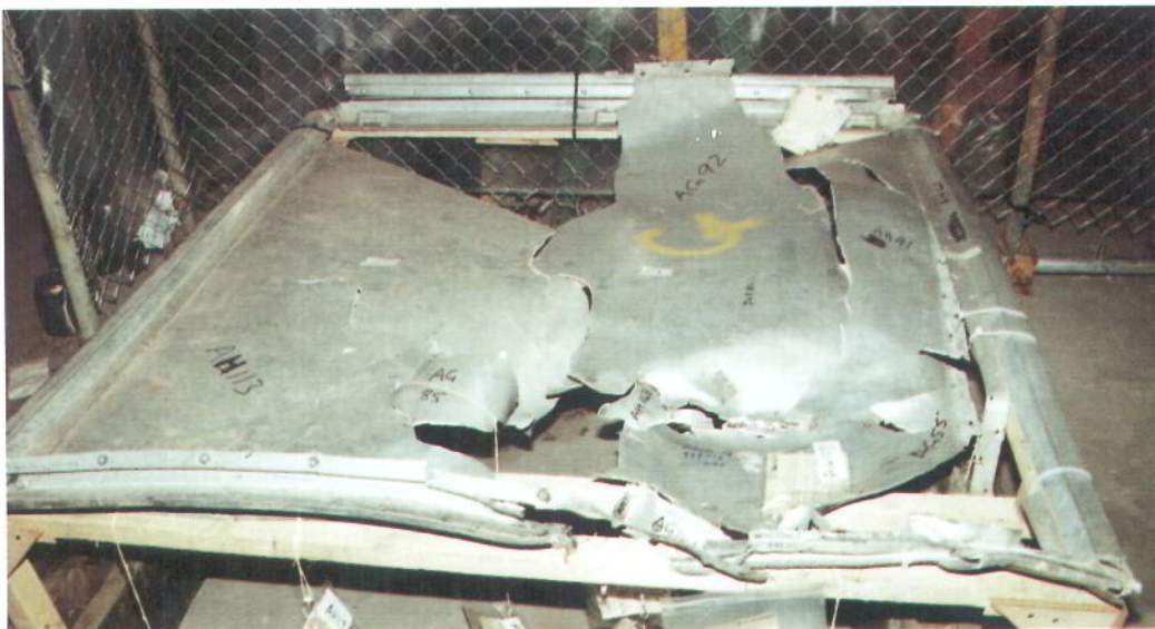
Detail of Damage to Container Floor
