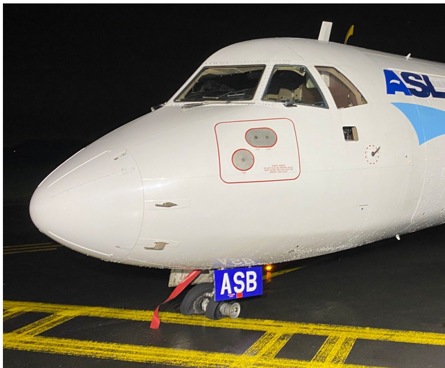
Figure 3 Damage to nose landing gear after landing
