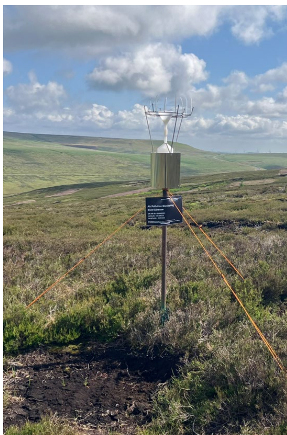
Figure 2. An example of a bulk rain collector (Moorhouse).
