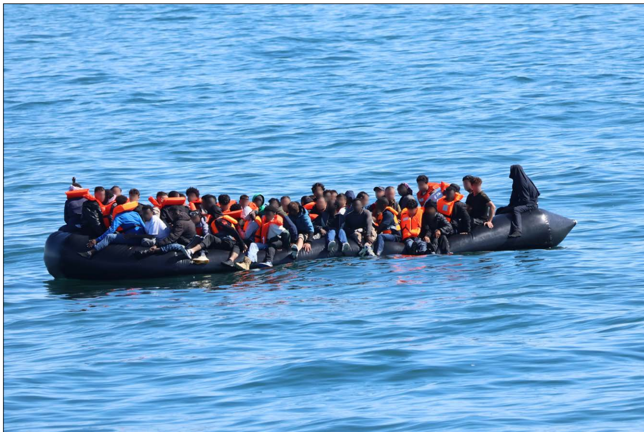
Figure 8: Migrant boat 512 during the initial approach, showing deflation and low freeboard
