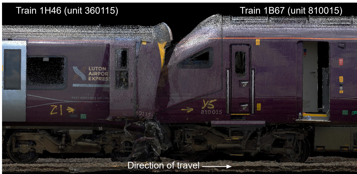
Figure 7: Side view of the collision (image created from laser scans).
