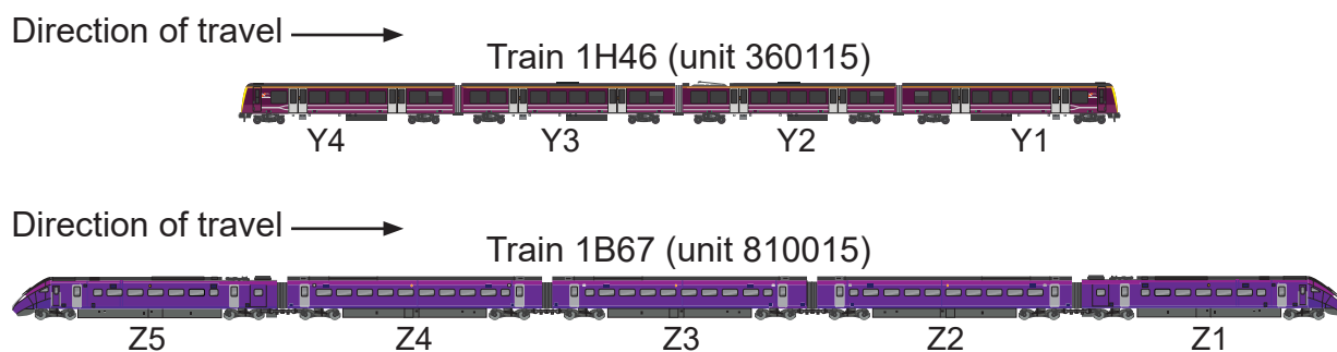
Figure 3: Formation of trains 1H46 and 1B67. The Y and Z numbering system was assigned by RAIB after the accident to assist with identifying vehicles.
