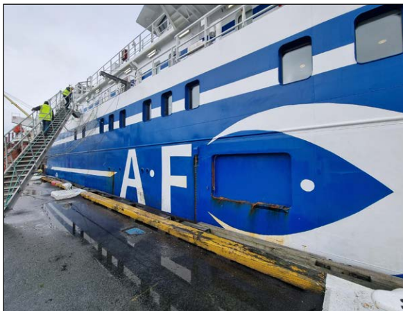
Figure: Line hauling hatch similar to that of Argos Georgia *
