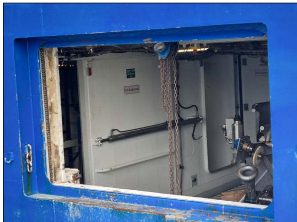
Figure: Line hauling hatch similar to that of Argos Georgia *
