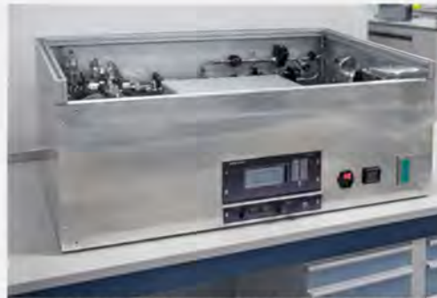
Plasma generating unit currently used for RIPPLE breadboard testing [3]
