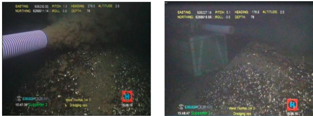
Figure 3-5 Photos of hose discharge and accumulation of cuttings at discharge point
