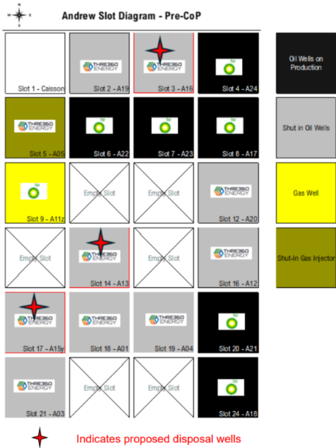
Figure 2-1 Andrew platform and Subsea Well Slot Diagram 8
