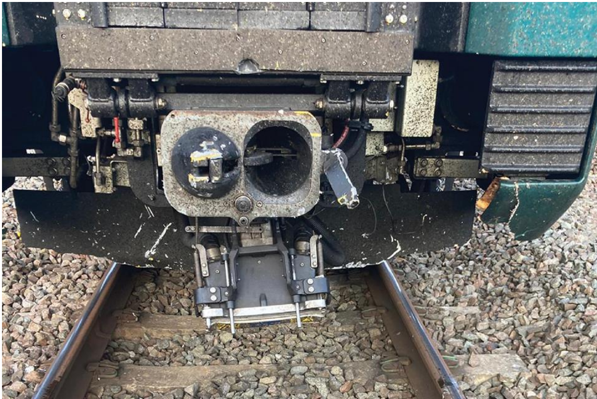
The damage to the front of the train (courtesy of Network Rail).
