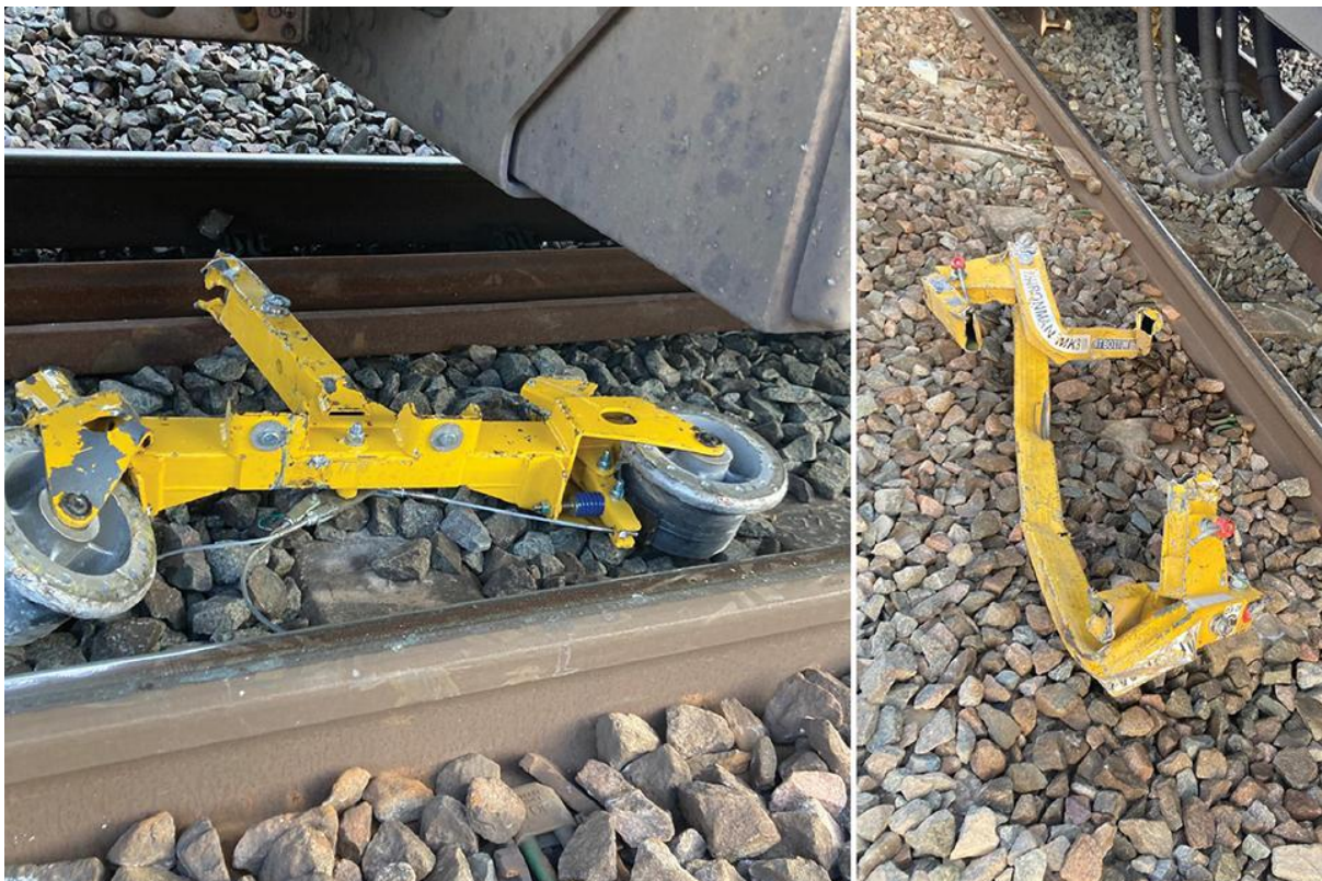
The remains of one of the MPRHs after the collision (courtesy of Network Rail).
