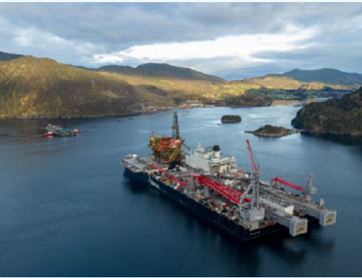
▲ Eider topside removal and TFS movement to Norway for disposal
