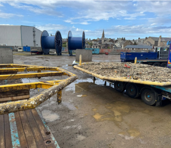
▲ Braemar and Devenick subsea roof panels following removal during Central North Sea Subsea Disconnections, awaiting cleaning at the scrap merchant, Peterhead, Scotland
