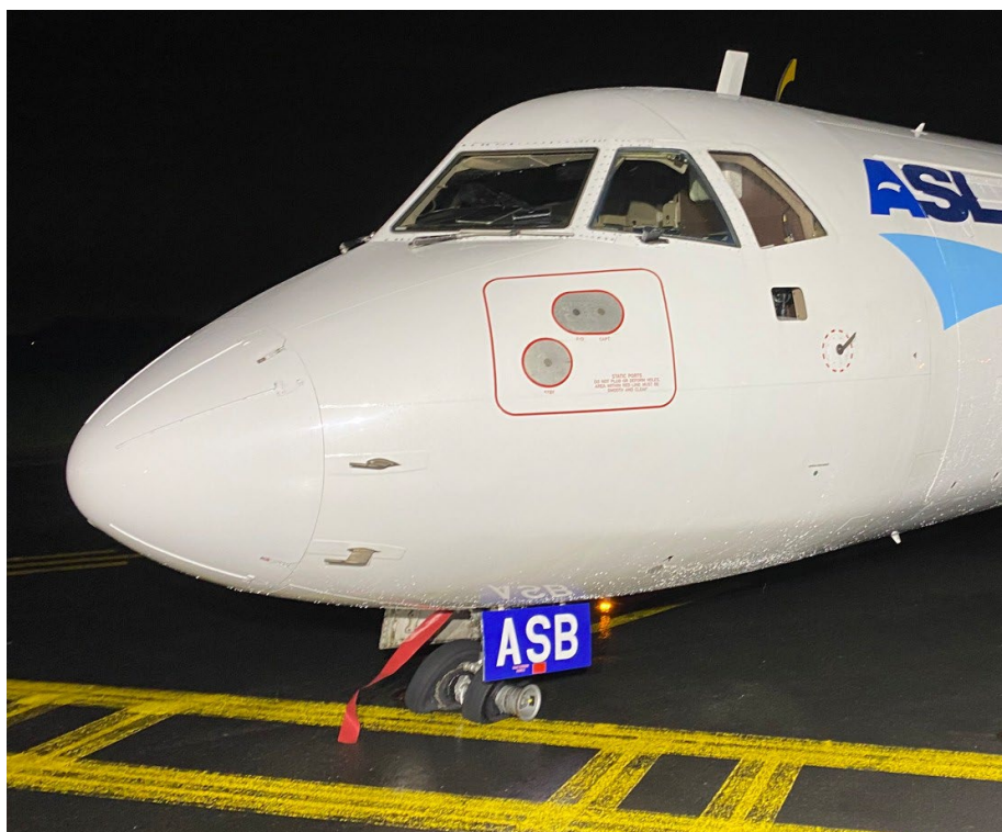
Figure 3 Damage to nose landing gear after landing
