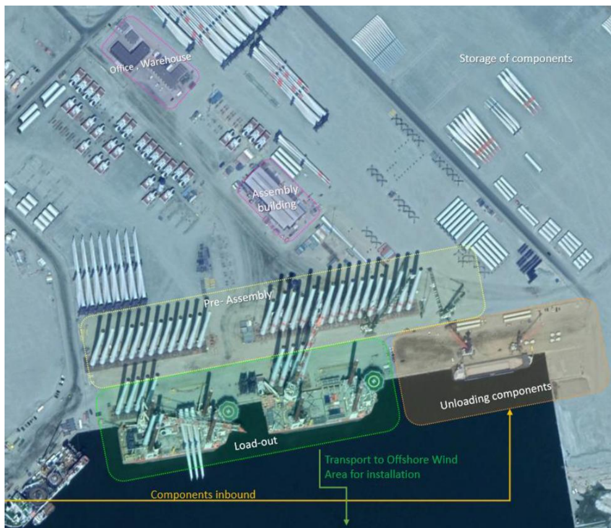
Figure 13: Illustration of sections at a marshalling port, the Port of Esbjerg in Denmark. [29]
