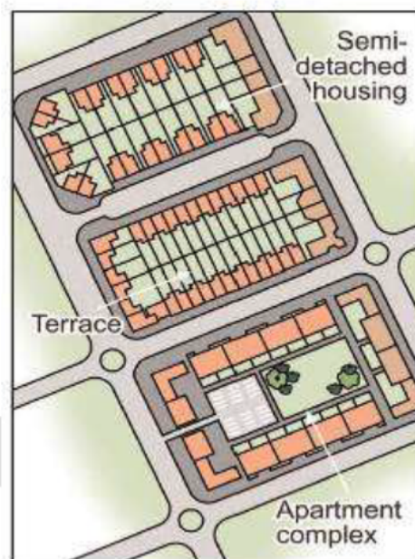
Figure 2.5: Perimeter blocks accommodate different building typologies which all fit in with the built form of surrounding development.
