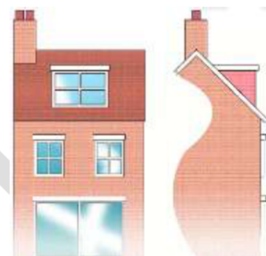
Figure 2.45: Position of dormer within the roof slope (explanatory example only).
