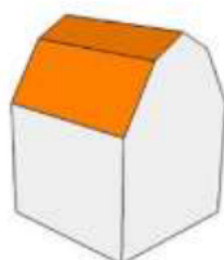
Figure 2.25: Gambrel roof ( http://www.geograph.org.uk/article/Roof-Types#mansard )
