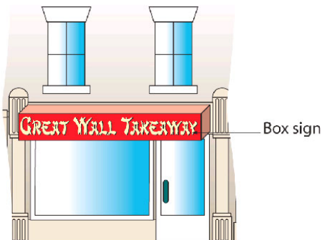
Figure 8: A box sign.
