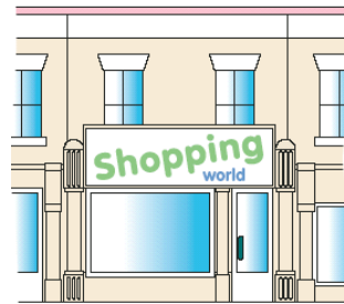
Figure 2: A disproportionate fascia board.
