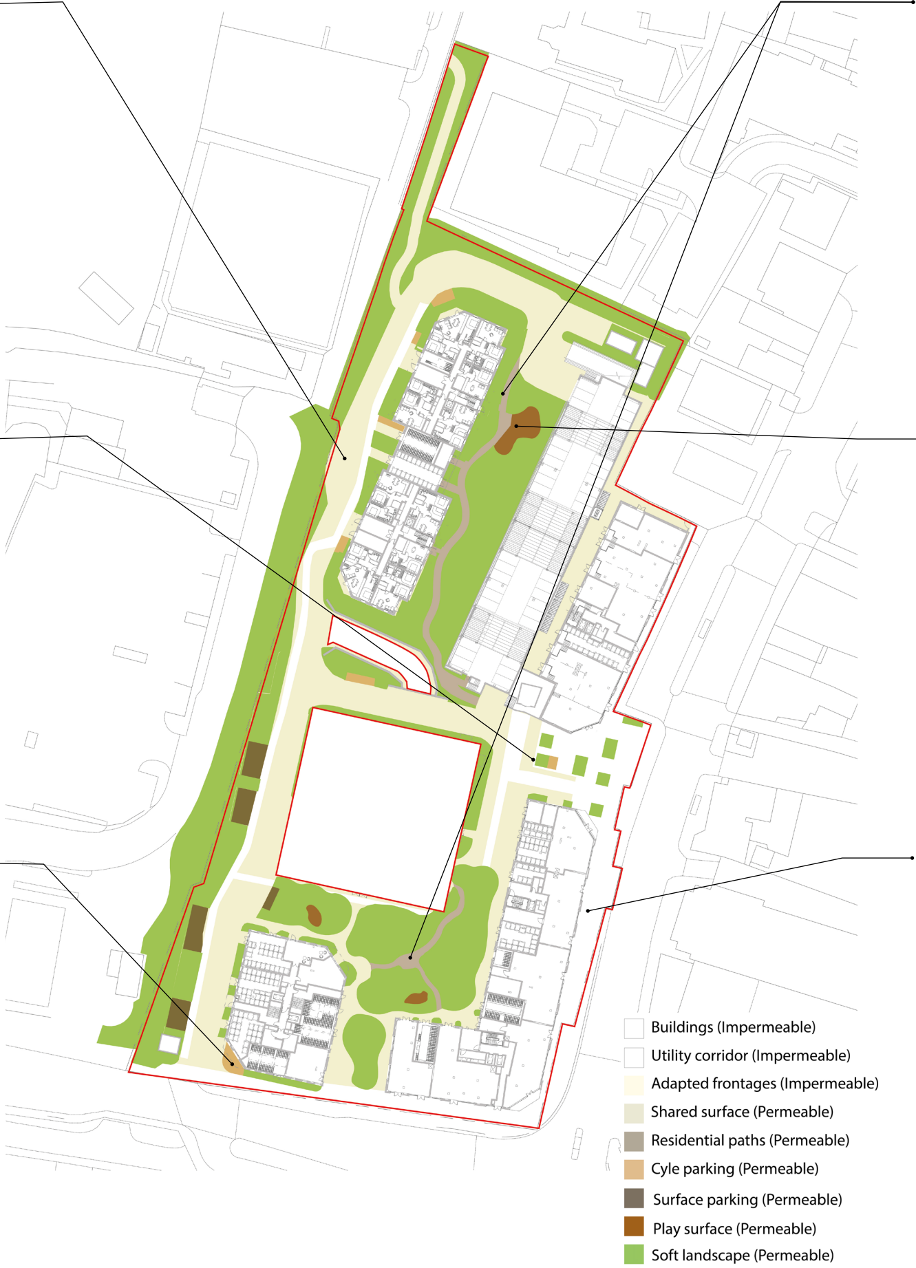
Private communal paths to be permeable block paving (south) and resin-bound gravel (north) with a brick border to provide a softer appearance and reference the brick facades
