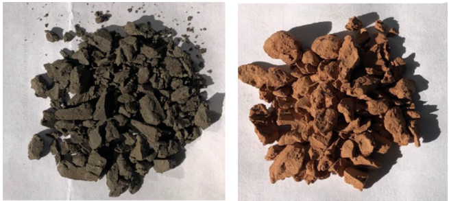
London Clay structure and colour
