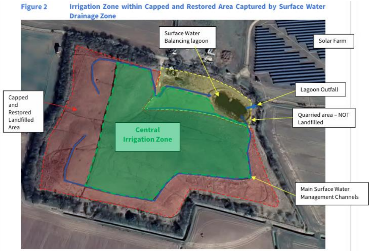
Figure 2 - Irrigation Zone within capped and restored area captured by surface water drainage zone
