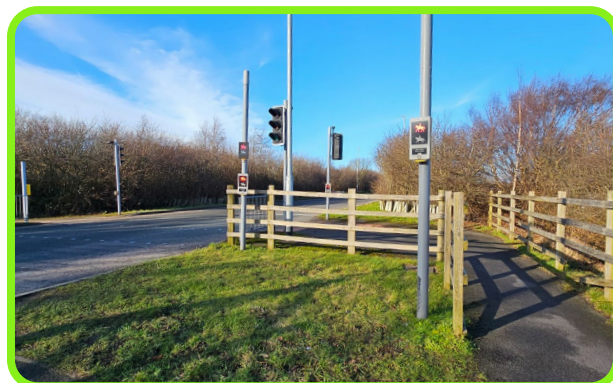
Figure 9: Uncontrolled crossing point with bollards, fence and wayfinding.
