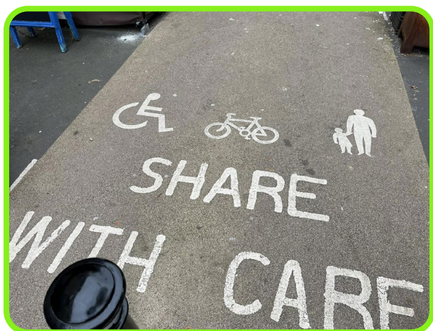
Figure 12-25: Simple non-prescribed surface marking to raise awareness of different path users sharing the space.
