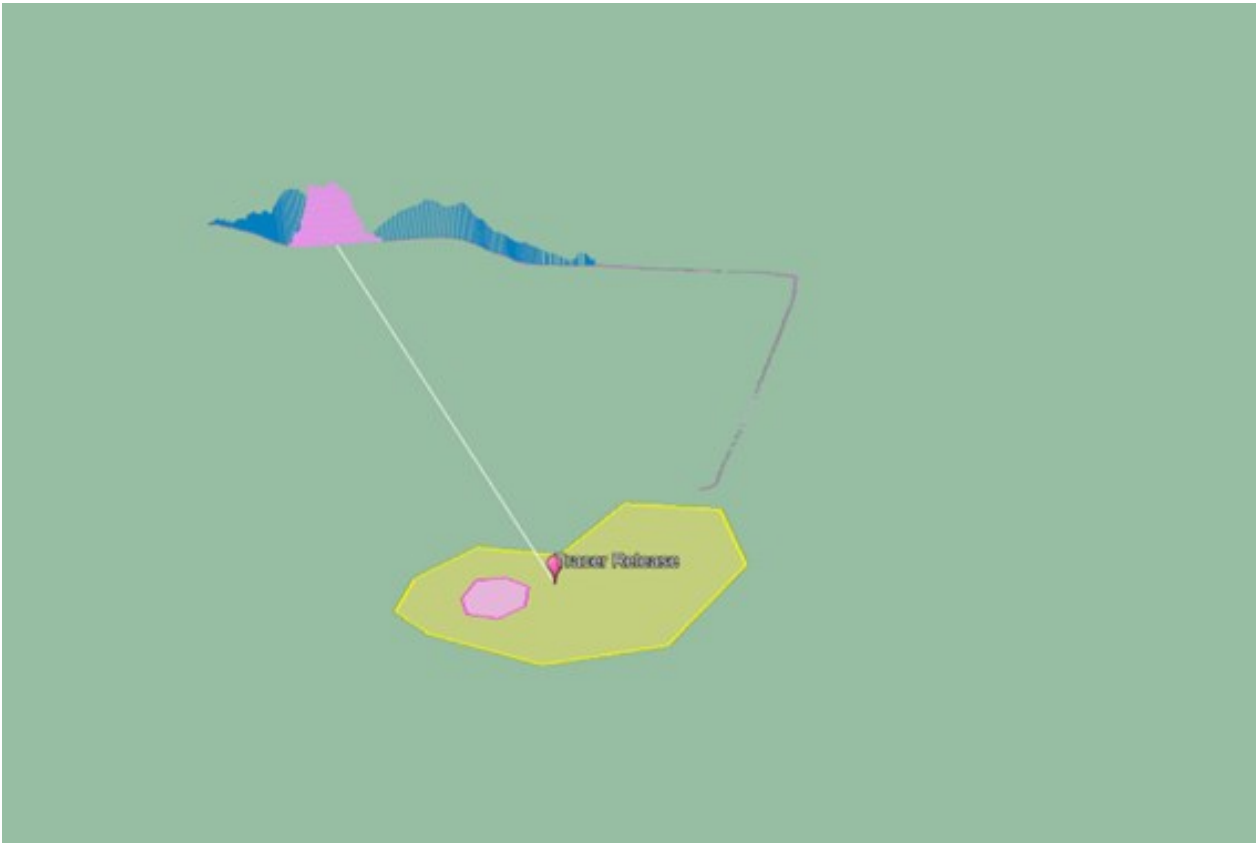
Figure 8.4: Methane and tracer gas concentration measured during Survey Y2_T3, 14/01/25
