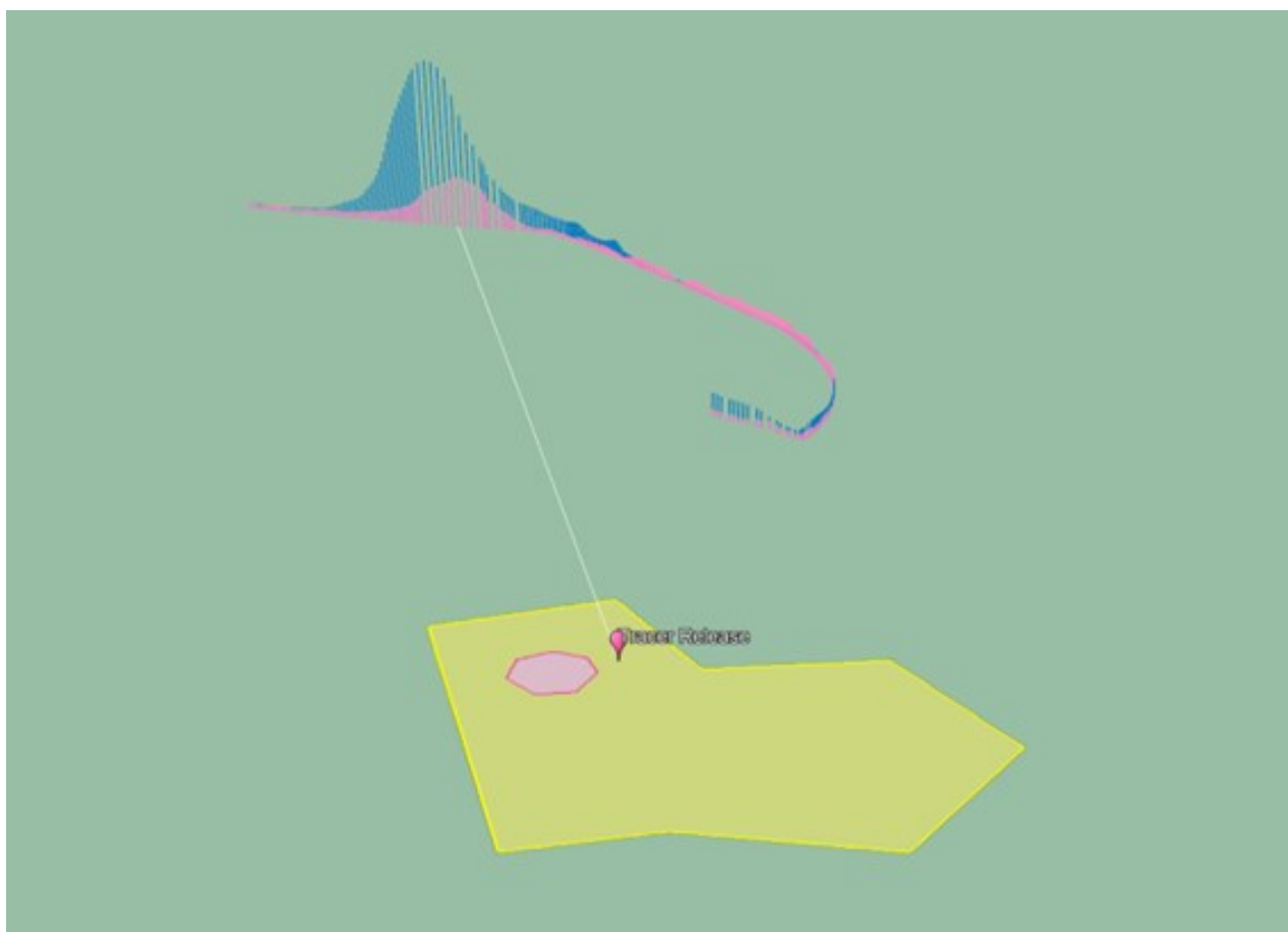
Figure 8.3: Methane and tracer gas concentration measured during Survey Y2_T1, 05/12/24
