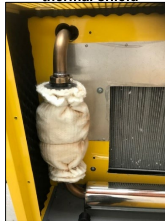
Figure 9. Catalytic converter is in a cloth thermal shield
