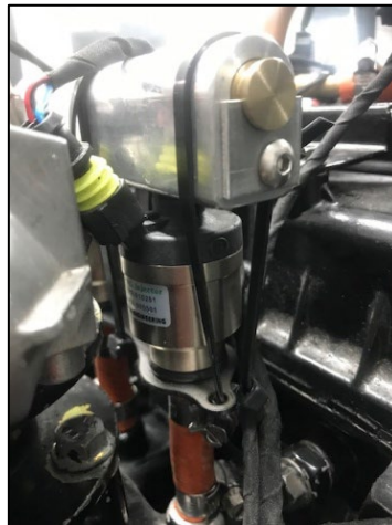
Figure 5. Hydrogen/LPG fuel injectors installed in inlet manifold
