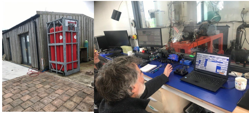
Figure 2. Test cell hydrogen store and control room
