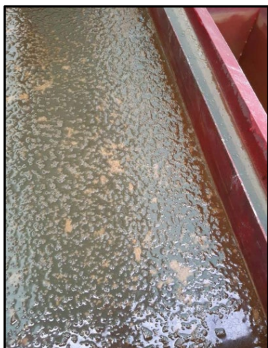
Plate 1. Oily sheen and emulsified product frequently observed in OWS (30.03.2022)
