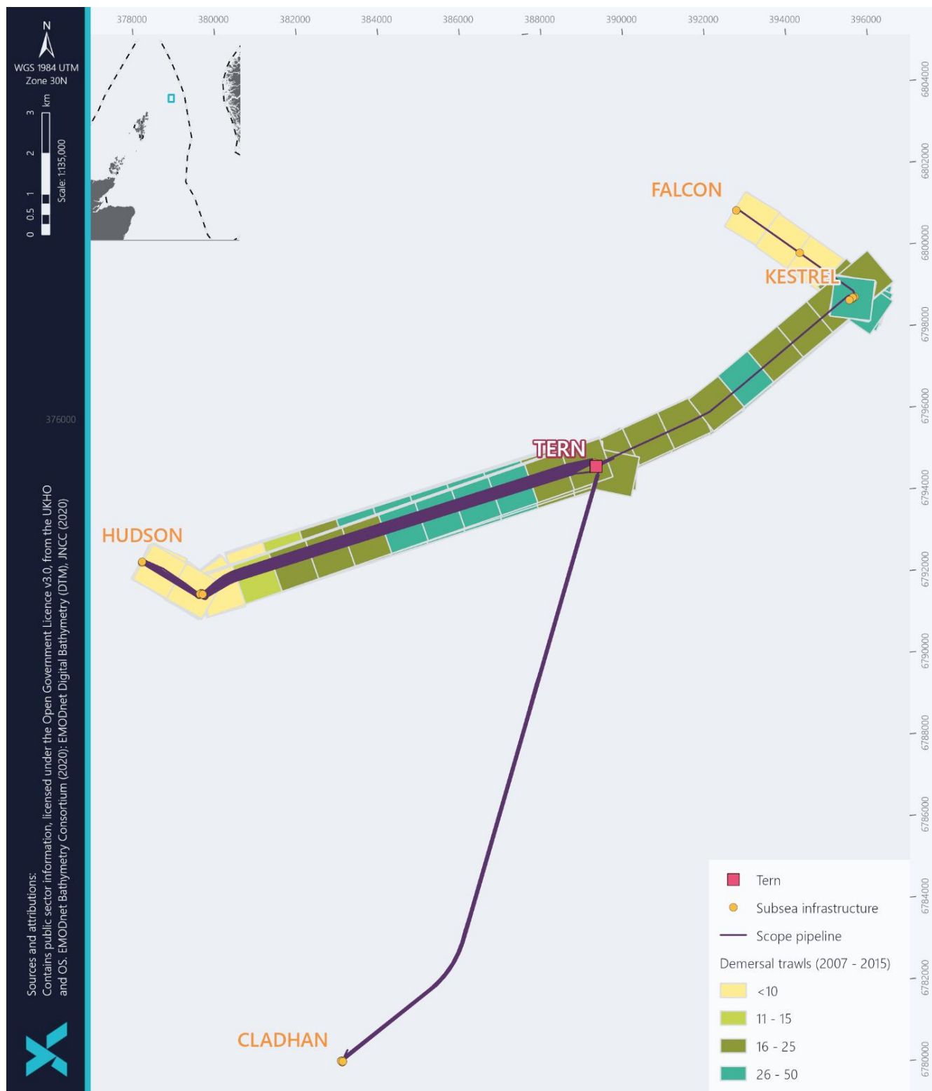
Figure 6-4 Trawling Across The Tern Area Pipelines
