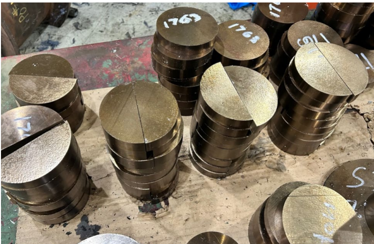
Figure 24: Depleted uranium after being cut into a mixture of quarter and half pucks
