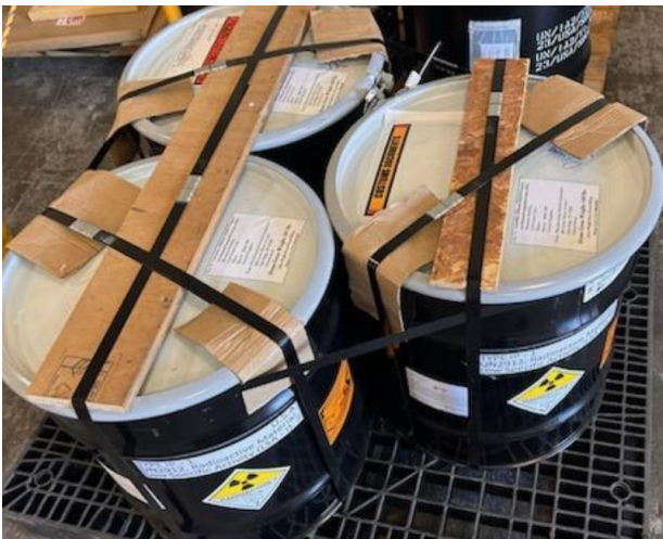
Figure 25: Drums containing the depleted uranium for shipping
