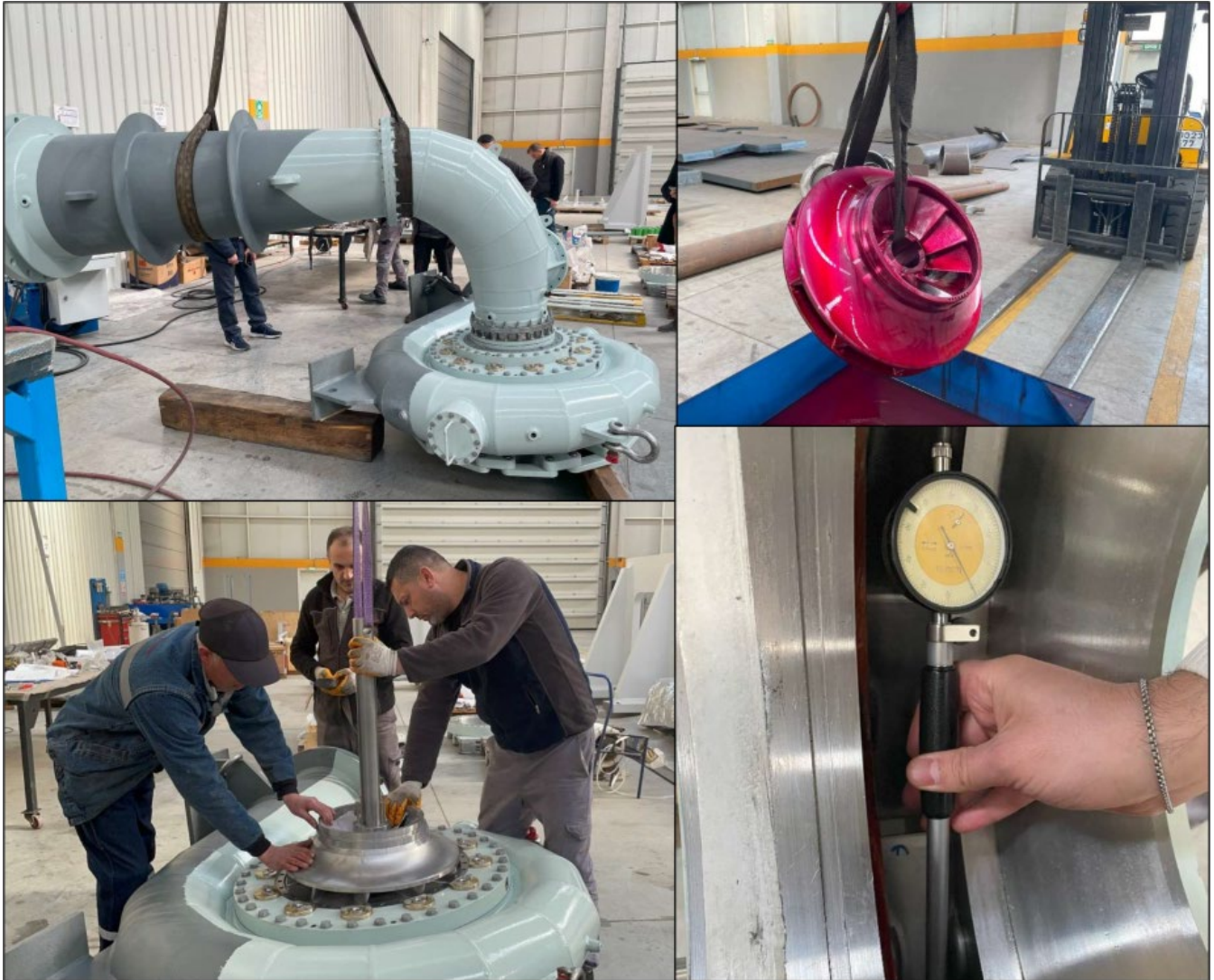
Figure 10 Turbine Factory Acceptance Testing
