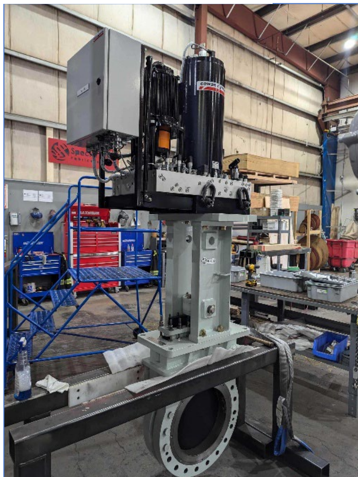
Figure 12 Main Inlet Valve (MIV) Factory Acceptance Tests
