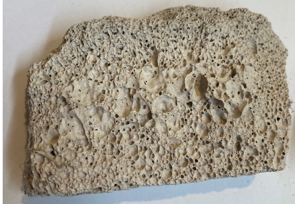
Figure 2: A fragment of RAAC showing its 'bubbly' appearance
