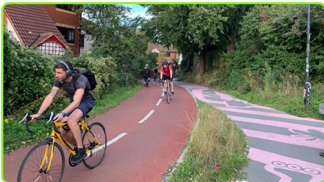
Figure 4-1: The Bristol and Bath Railway Path is mostly a 3m shared use route, but separates users at busy sections.
