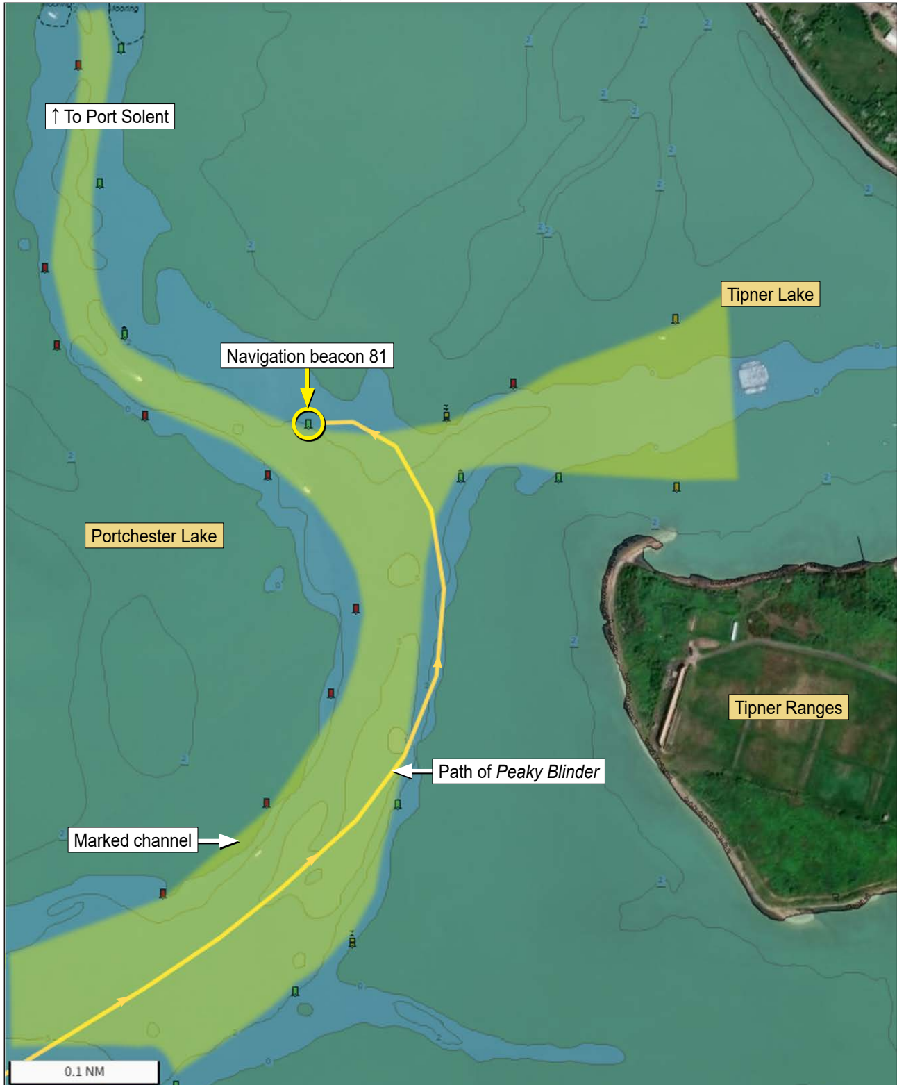
Figure 3: Departure of Peaky Blinder from the marked channel
