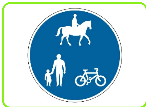
Figure 12-9: Sign 956 – Route for use by pedal cycles and pedestrians only.
