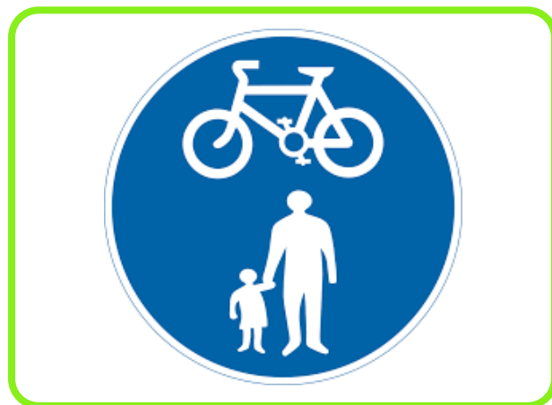
Figure 12-9: Sign 956 – Route for use by pedal cycles and pedestrians only.
