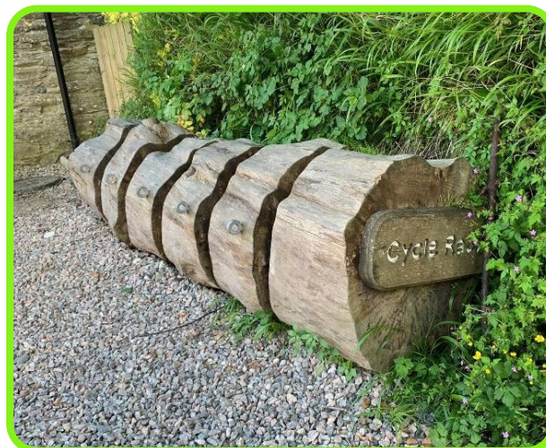
Figure 11-10: Rural cycle parking that fits in a rural setting but is not secure.
