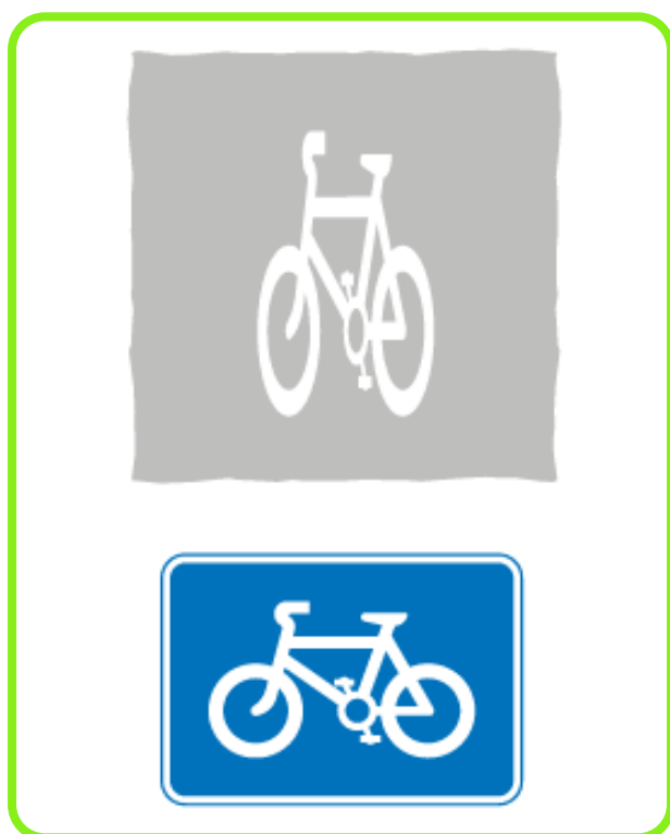
Figure 12-1: Road marking to diagram 1057 and traffic sign to diagram 967.
