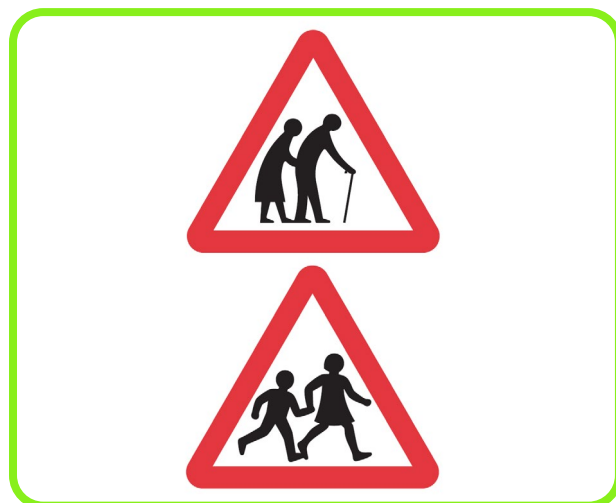
Figure 12-12: Signs warning of frail or disabled pedestrians (diagram 544.2) and children (diagram 545) crossing ahead.
