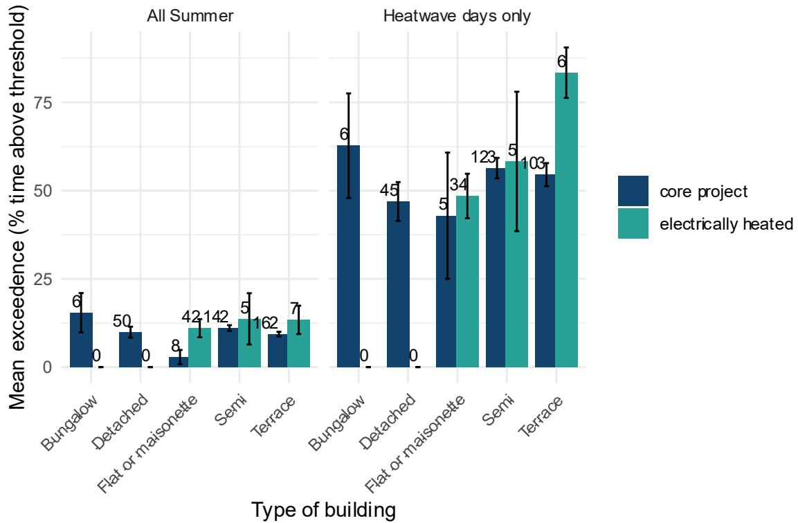
Figure 8: Variation in mean exceedance in daytime (adaptive threshold) across different types of building (error bar indicates confidence interval of +/- standard error of mean). Data analysed for 'All Summer' (2025) and 'Heatwave days only' (2025).
