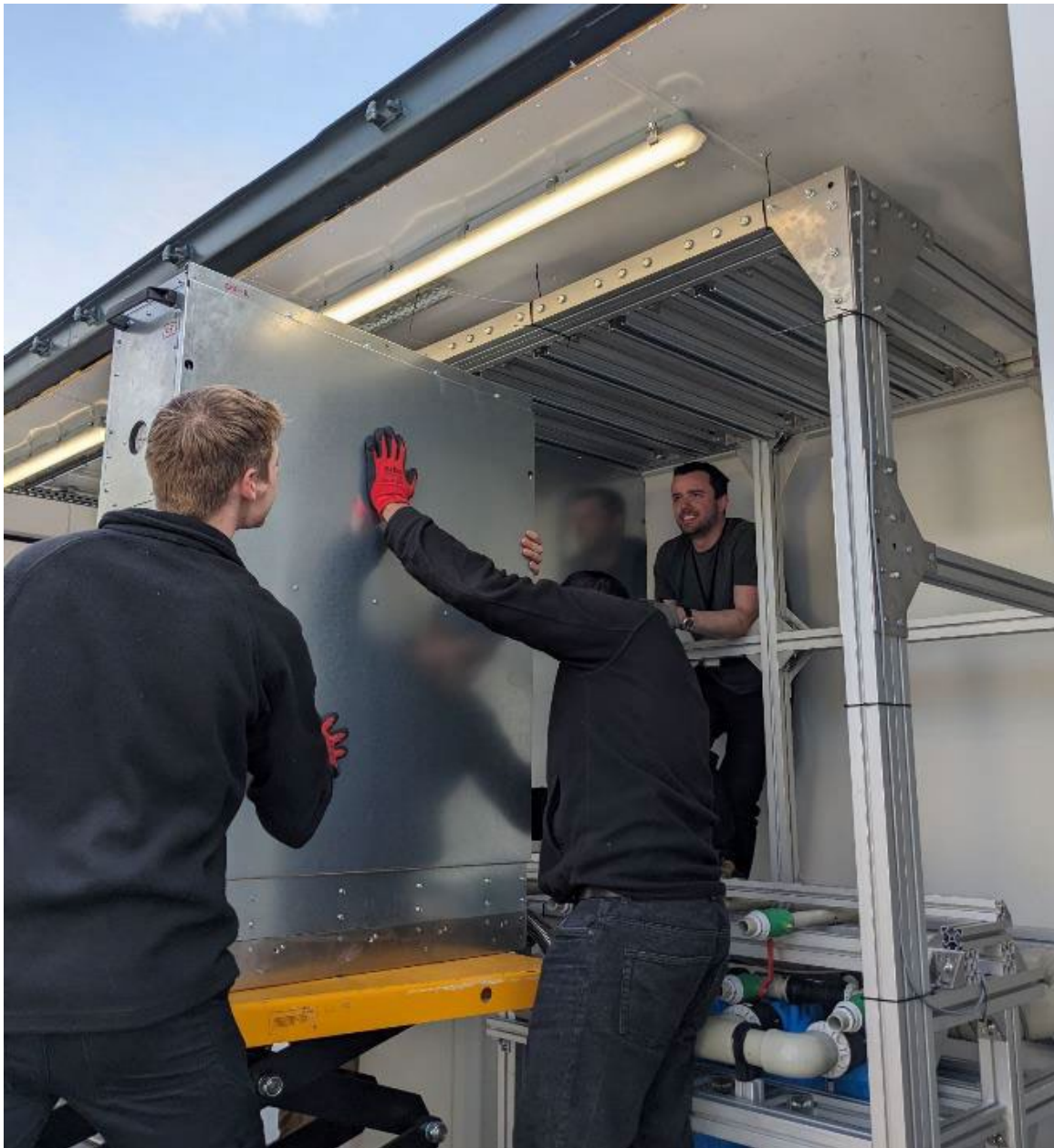
Figure 3: A complete pack assembly being mounted into the test system
