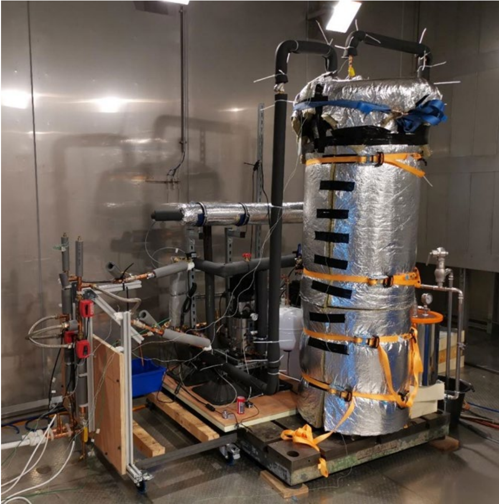
Figure 61: The TCS unit, including ancillary equipment, located within the environmental chamber.
