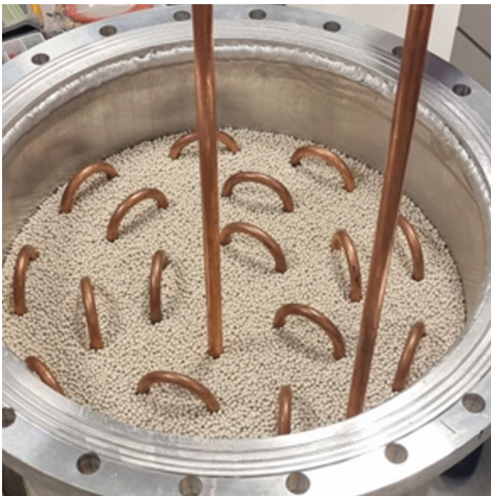
Figure 49: Gen 2.1 vessel, heat exchanger and TCS material.
