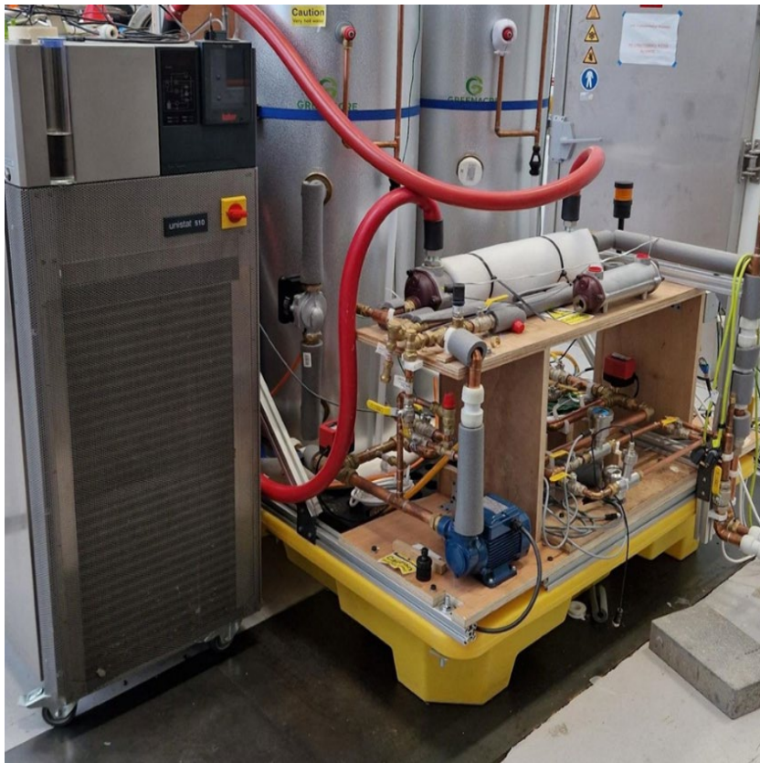
Figure 22: The thermal testing rig at LVV, with the Huber 510 thermoregulated supply unit shown on the left.
