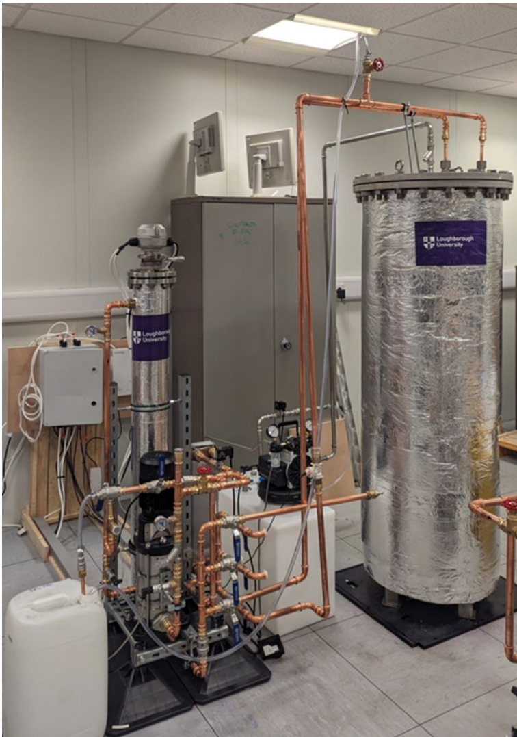
Figure 38: A Gen 1 TCS vessel connected to heating system and controller at CREST.
