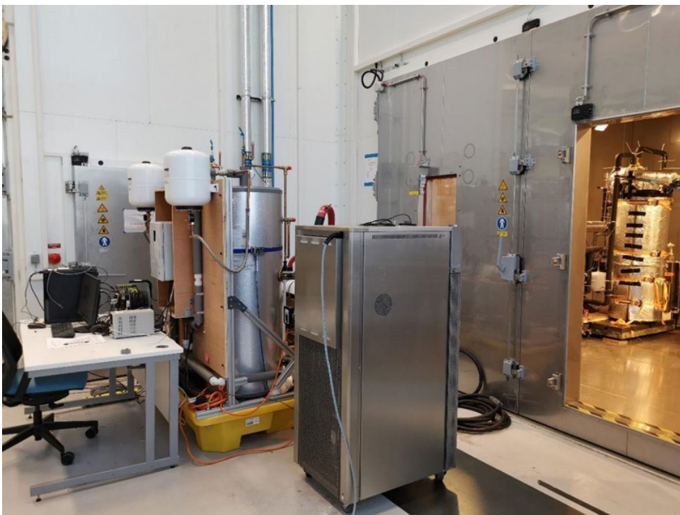
Figure 59: The full test rig set-up for TCS testing
