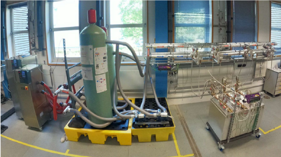
Figure 7: A three module PCM store under test at CREST thermal store test facility.
