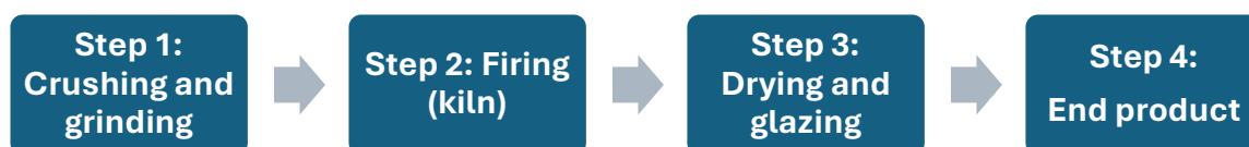
Figure 5: Main production steps for Ceramics manufacturing
