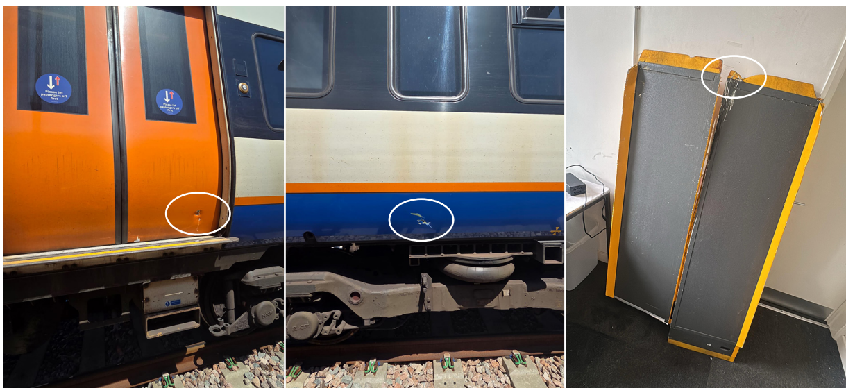
Figure 3: Damage (circled) to a door on train 9D18 (left), to side panelling (middle) and the portable access ramp (right) (courtesy of ARL).
