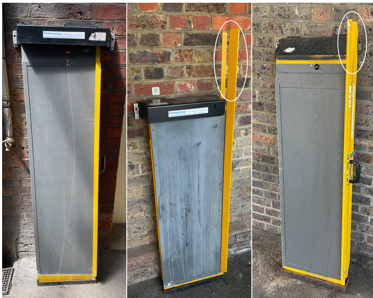
Figure 13: Portable access ramps shown stored in their folded condition, on the left for a class 377 (which was also designed to work on class 455 trains that are now out of service), in the middle for a class 700 (door closure prevention arms circled), and on the right for a class 378 (door closure prevention arms circled).
