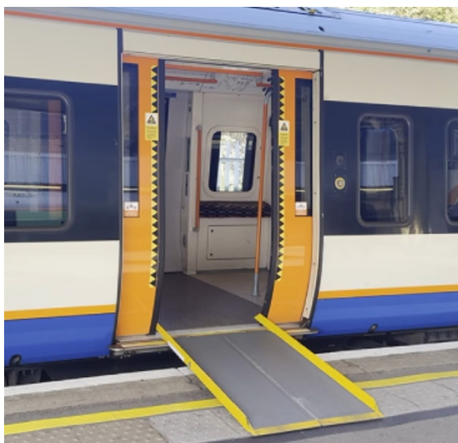
Figure 14: Door closure prevention on a class 378 electric multiple unit with correctly specified portable access ramp (courtesy of ARL).
