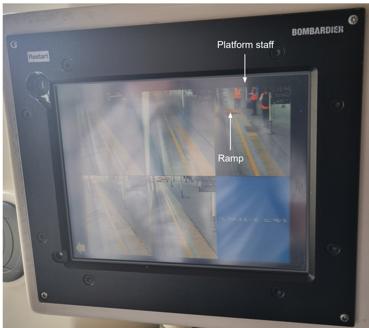
Figure 24: DOO monitor in cab of a class 378 unit from a reconstruction at Norwood Junction station showing a portable access ramp attached to car 3 and platform staff.
