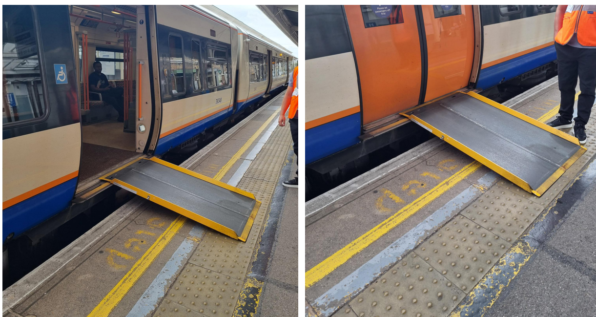
Figure 15: Reconstruction of the fitment of a class 377 portable access ramp to a class 378 unit (courtesy of ARL).
