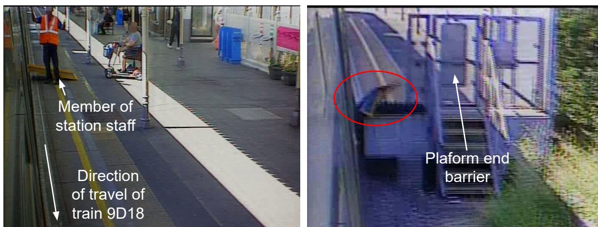
Figure 2: Portable access ramp attached to train 9D18 as it departed Norwood Junction station (left), ramp (circled in red) impacting the barrier at the end of the platform (right). Images are derived from the bodyside CCTV cameras fitted to the train (courtesy of ARL).
