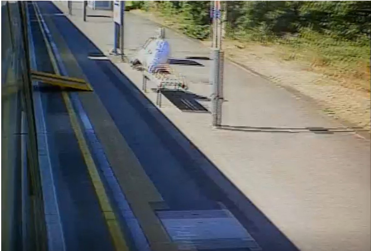
Figure 8: Member of public having moved their legs out of the way of the moving portable access ramp (courtesy of ARL).
