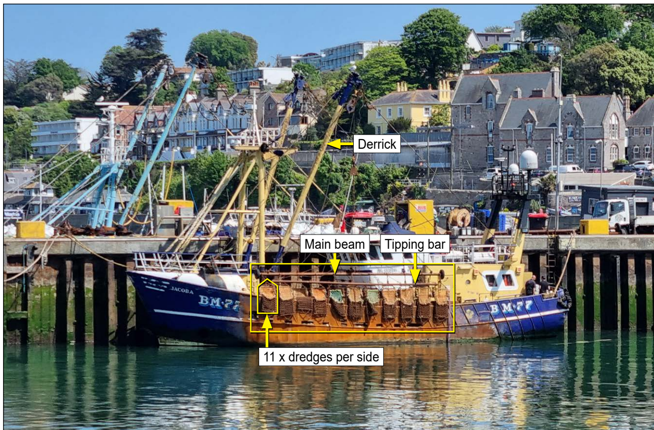
Figure 4: Jacoba alongside, showing the configuration of the scallop dredges
