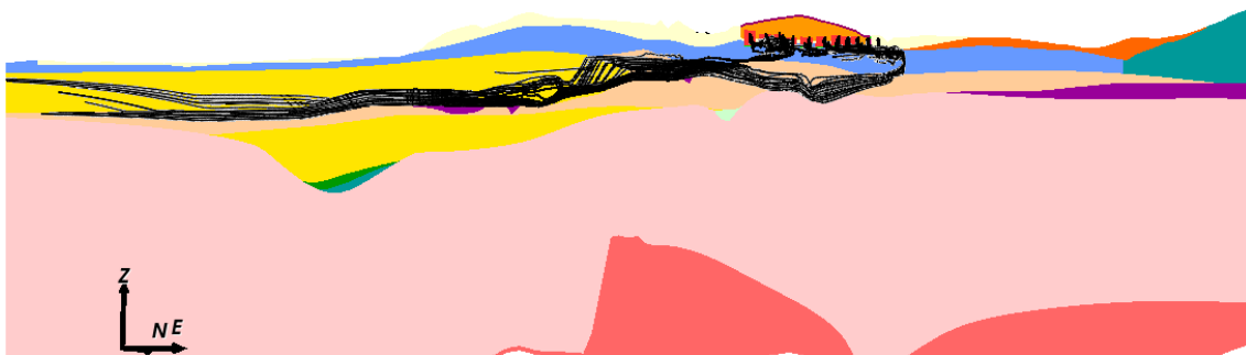
Figure 5.8 Section view of pathlines from starting positions in the trenches shown passing through the lithofacies units (blue is B2, bright yellow is B3SS, light brown is B3), vertical exaggeration 5:1, for the 2025 hydrogeological model 10
