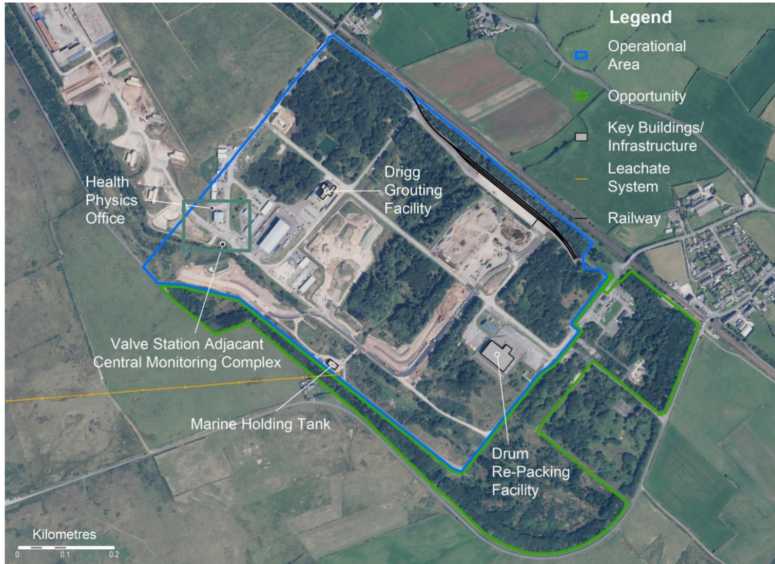
Figure 5.2: LLWR Operational and Opportunity Areas – main infrastructure (the figure does not show the drainage lines of the leachate management system that lead to the MHT – see ' Engineering Design ' report [5])
