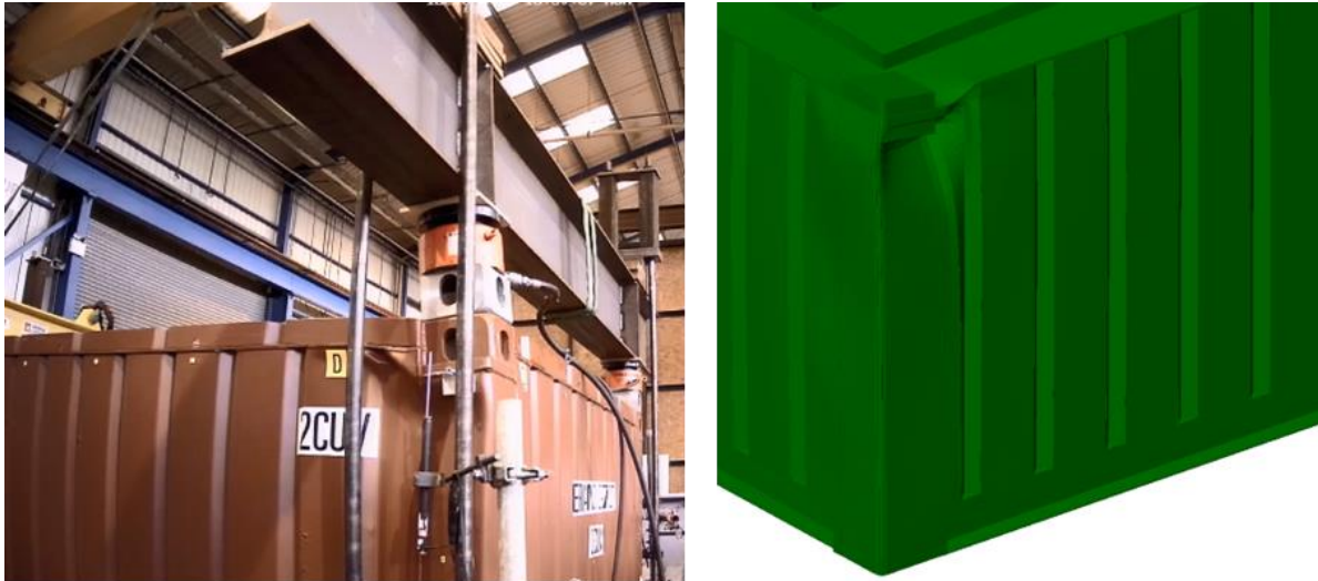
Figure 5.3: Physical testing of containers, and corner element deflection analysis in finite-element models. The photograph and model outputs are indicative of the broader physical testing and finite-element analysis outcomes presented in [67] and supporting references.
