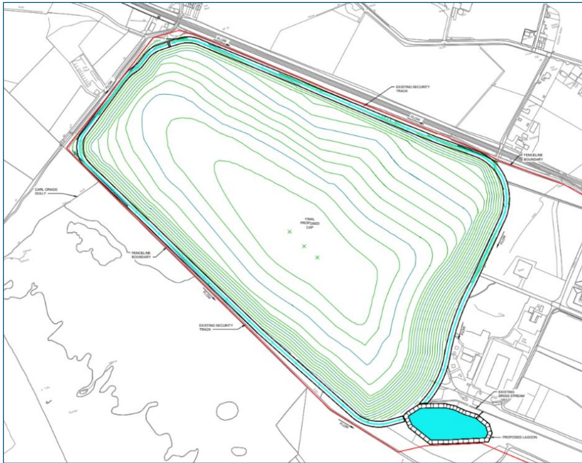
Figure 7.2: Final cap drainage
