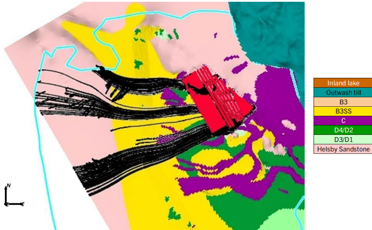
Figure 5.18: Surface view of the pathlines (in black) for the 2130 reference climate model overlaid over the deeper units. The approximate extent of unit B2 is shown in pale blue [24].
