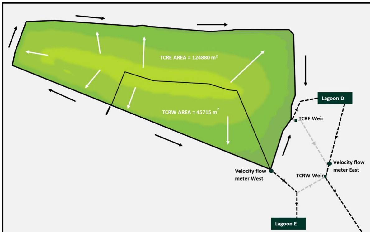
Figure 4.3: Trench cap catchment areas and relevant monitoring locations
