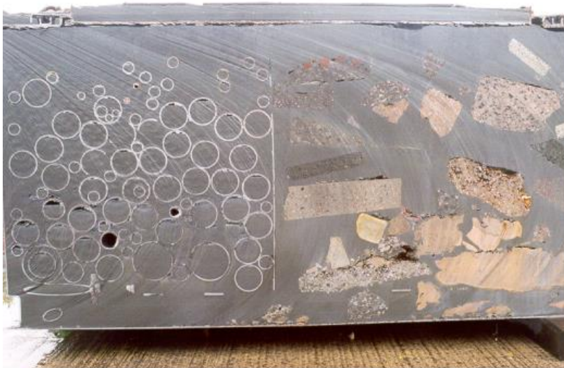
(b) Metal pipes, which are filled by cement grout, but with some enclosed void space (left), and concrete blocks (right)
