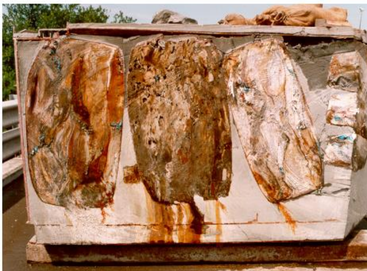
Figure 3.1: Photographs of sectioned test-grouted ISO containers, showing the distribution of grout, which fills most of the void spaces [20]
