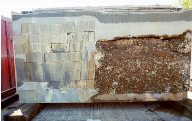
(a) Absorbent blocks (left) and soil/rubble (right), which shows little ingress and mixing of grout into the soil
