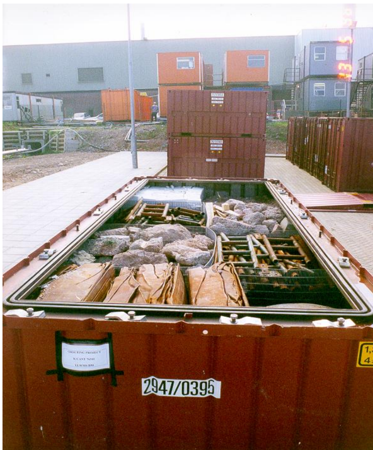
Figure 5.2: View of demonstration ISO prior to grouting
