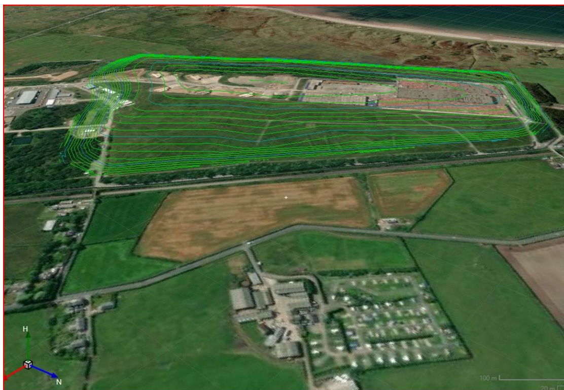
Figure 3.3: Contours of the final cap completed over Repository
