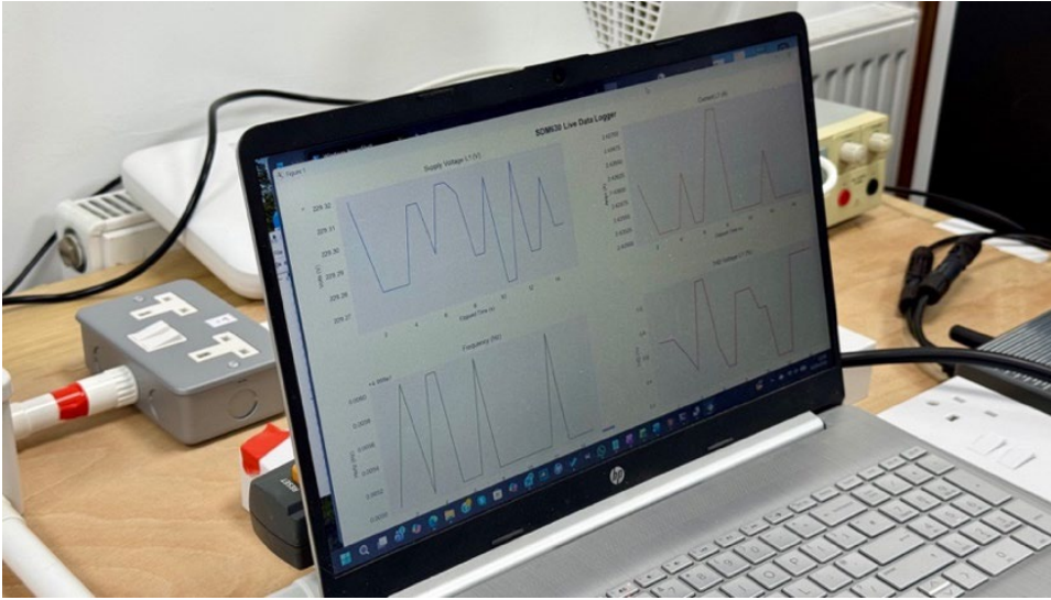
Figure C.3 Laptop capturing real time frequency tolerance results, Yate (© Arceio Limited)
