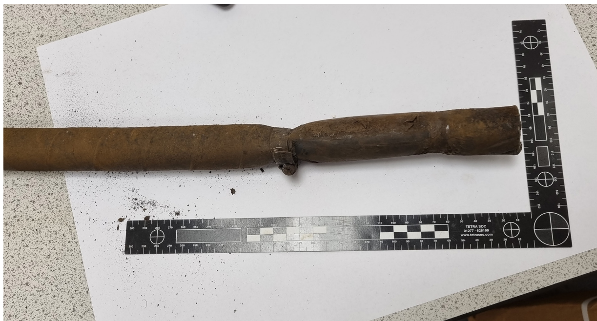
Figure C8: The sand hose taken from the driver's side of 57841. In this image, one of the hose clamps and the pipe clamp have been removed, leaving in place the deformed hose clamp.
