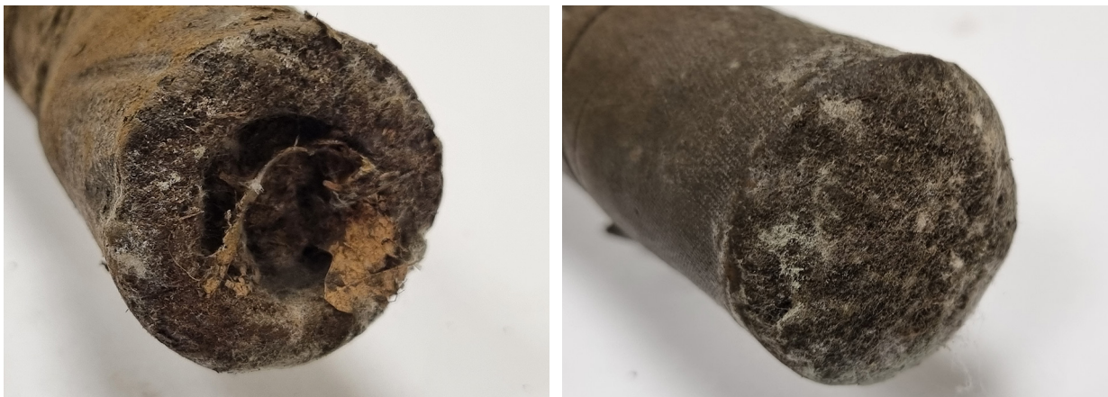
Figure D1: The blocked sand delivery hoses from leading vehicle 57841 during inspection.
