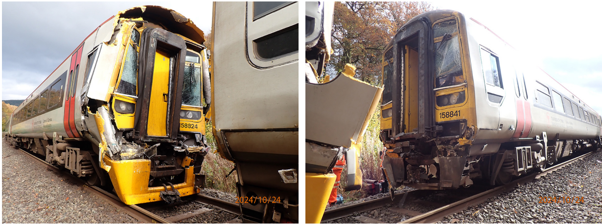
Figure 56: Damaged cab ends side-by-side on site (after separation) to show difference.
