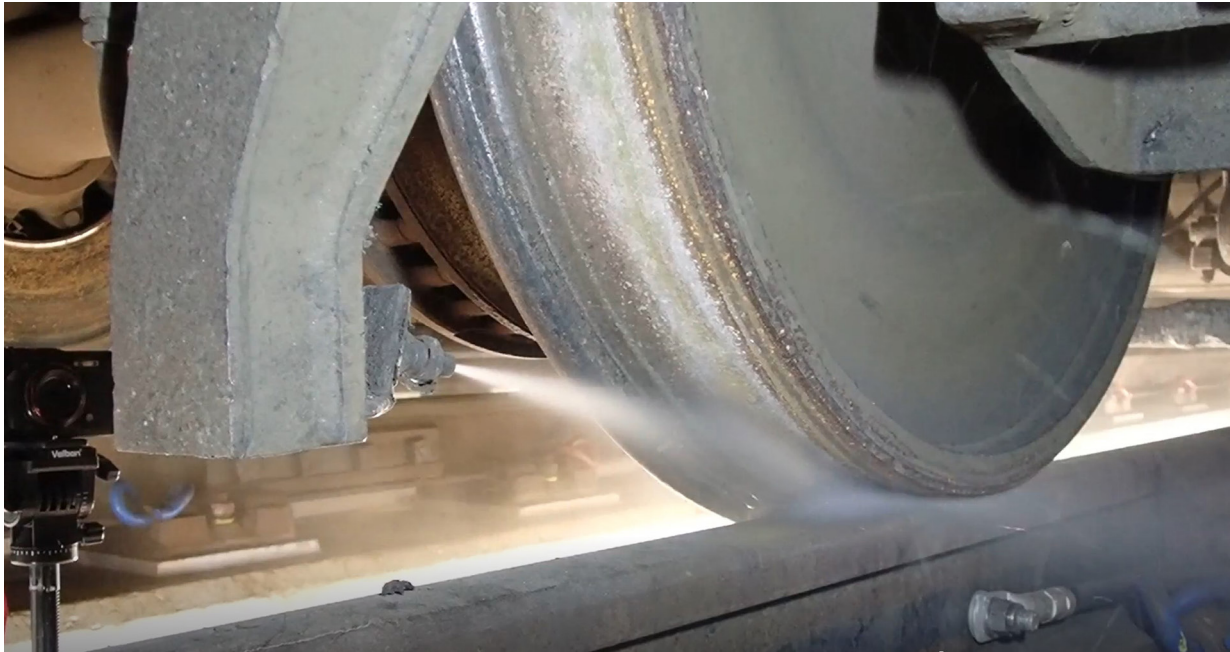
Figure 34: Emergency one-shot sander being deployed; note the powerful jet of sand.
