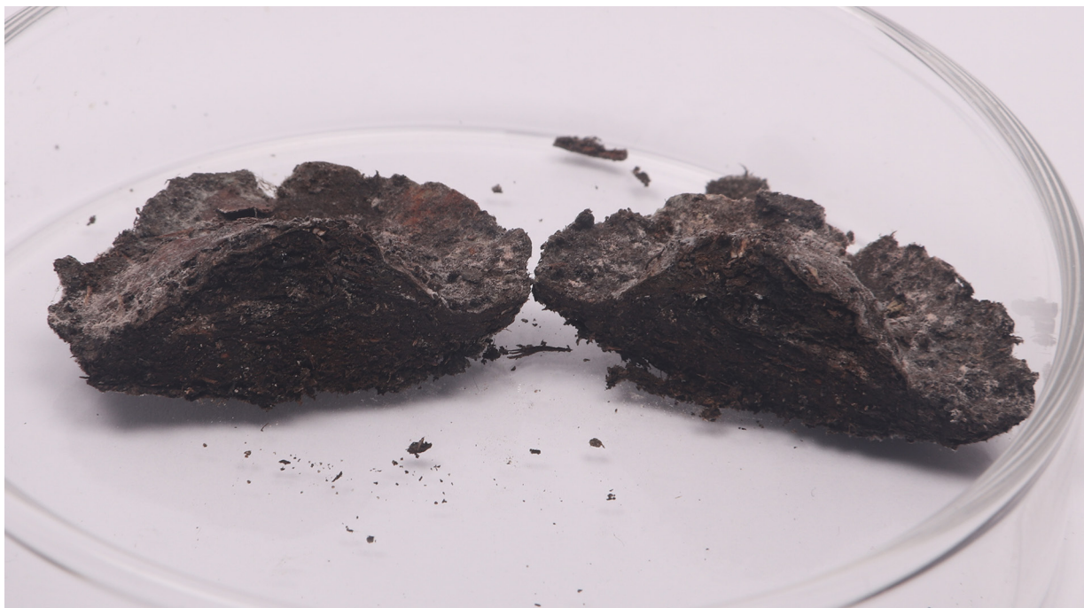
Figure D2: The plug of material from the end of the non-driver's side hose after being cut in half.
