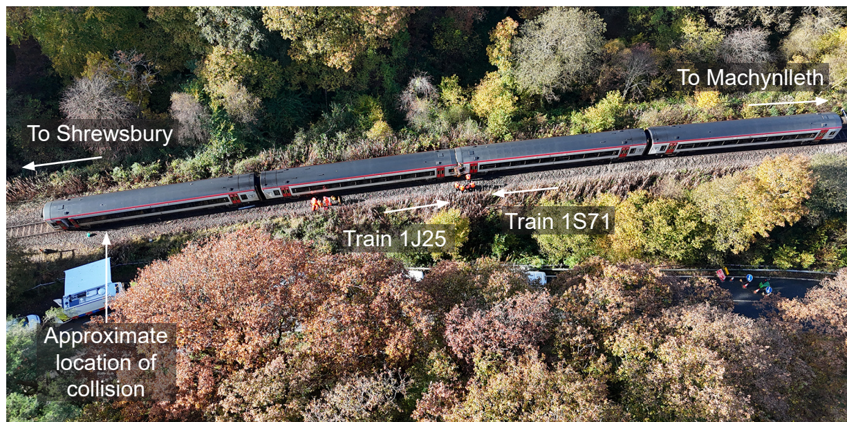
Figure 16: The trains involved, showing the approximate location of the collision and the final resting position.
