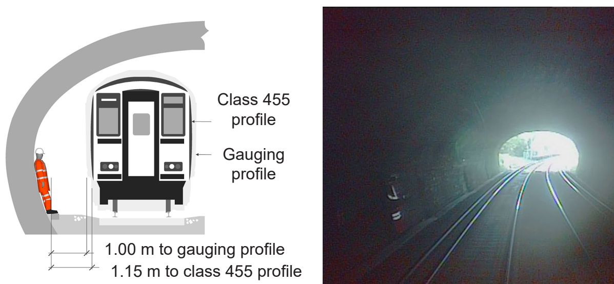
Figure 15: Position of track worker inside the tunnel as the train passed, based on gauging information from Network Rail (left-hand image) and from FFCCTV (right-hand image, courtesy of South Western Railway).
