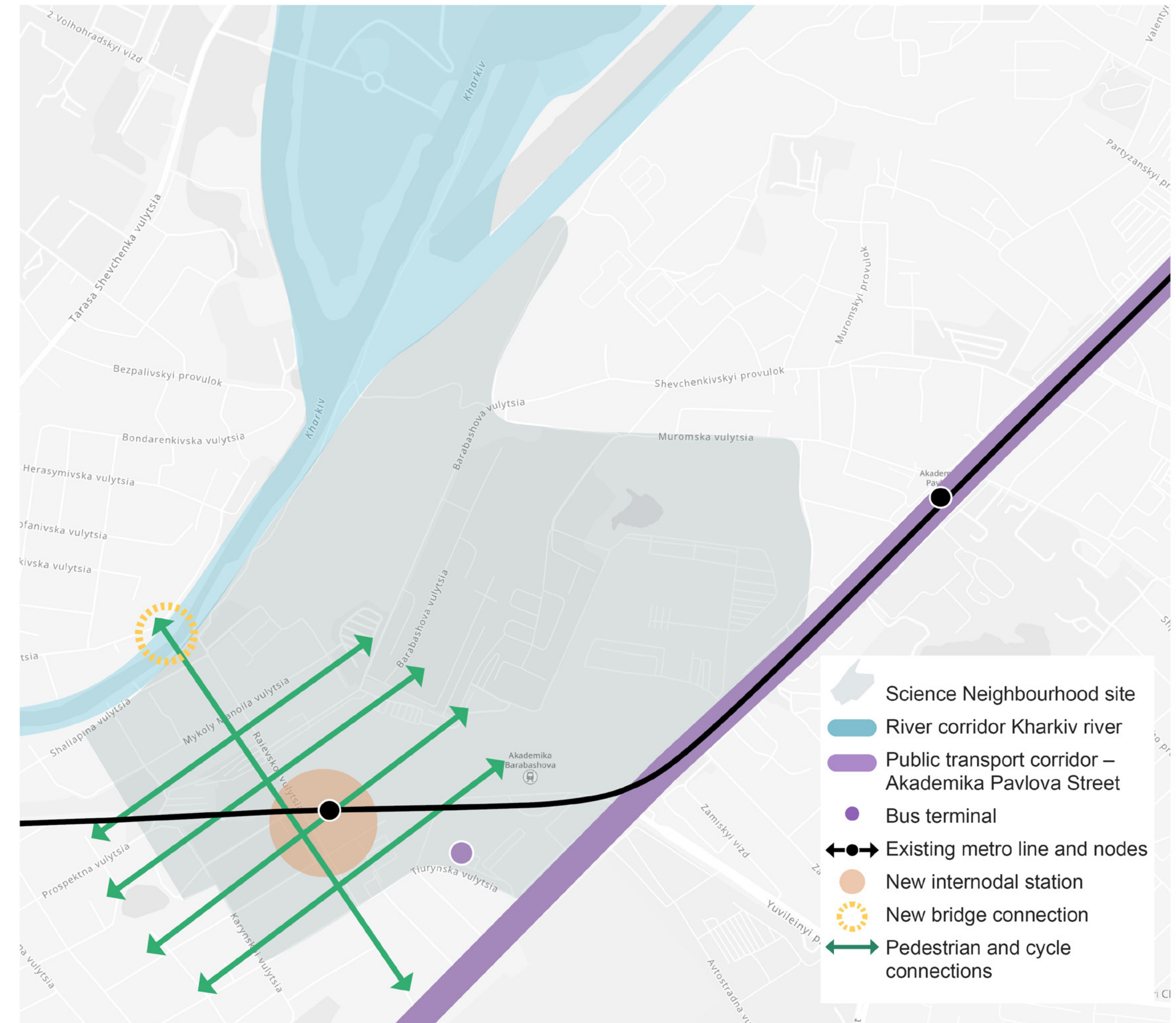
Figure 23 Project 3.2 - Kharkiv River Bridge - new active travel and public transport bridge connecting the science neighbourhood to city centre Source: Arup
