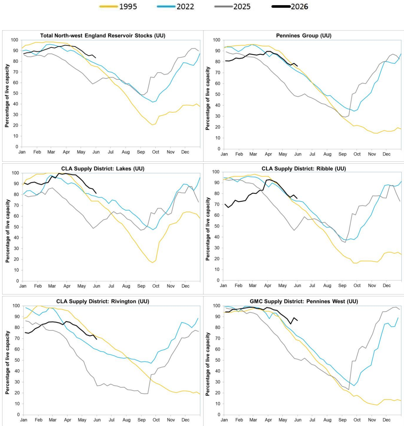
Figure 6.2: End of month reservoir stocks for supply districts across North-west England and selected individual reservoirs for current year (2025) and representative years: 1995, 2003 and 2022. Note: Historic records of individual reservoirs and reservoir groups making up the regional values vary in length.
